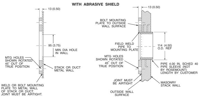
NOTE: ALL MASONRY STACK WORK AND JOINTS EXCEPT ADAPTOR PLATE NOT FURNISHED BY ROSEMOUNT.
